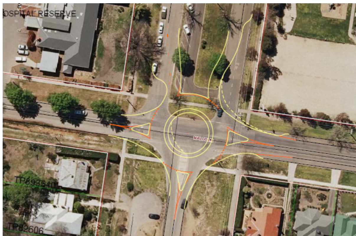
Figure 6.1.5: Proposed works at Malcolm Street/Highett Street intersection
