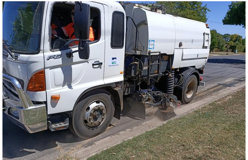
Street sweeping truck overhead suction boom being used to clean stormwater pits, and kerb sweeping reducing manual handling significantly for outdoor staff.
